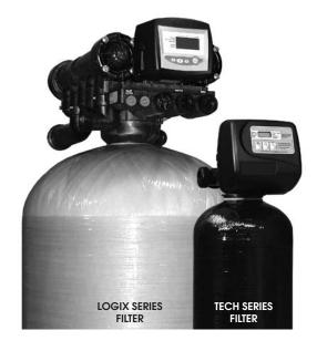
Safe Water Technologies' Commercial Sediment Filters are built utilizing SWT's FilterEase™ filter media. These filters are designed to remove ferric iron, silt, and turbidity, and are preferred when water flow rates and pressures are limited. Sediment filtration down to the 10 to 20 micron level is common. SWT takes care of the little extras such as: machined PVC distribution systems and anthracite underbedding to prevent channeling.
